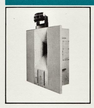
A high quality Duplex stage loudspeaker system comprising separate high efficiency units for bass and treble reproduction. The high frequency unit is designed to provide even distribution of sound over the whole auditorium. The low frequency assembly consists of two 15" direct radiators mounted in a matching baffle. The half section network provides for cross-over at the optimum frequency
