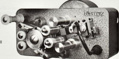
projector. These are rugged double-drum pull-through scanning mechanisms for magnetic reproduction and incorporate a free-running composite sprocket for 35 or 70mm film and easily interchangeable single, four or six track plug in magnetic head assemblies.
