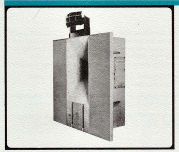
A high quality Duplex stage loudspeaker system comprising separate high efficiency units for bass and treble reproduction. The high frequency unit is designed to provide even distribution of sound over the whole auditorium. The low frequency assembly consists of two 15" direct radiators mounted in a matching baffle. The half section network provides for cross-over at the optimum frequency.
