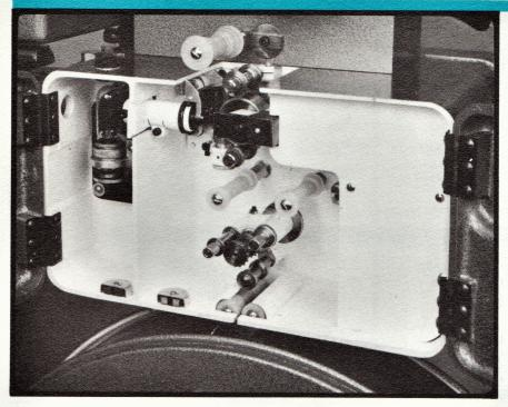
For use with 35mm Single Photo Sound Track Film. This reproducer employs a photo voltaic cell giving greatly improved signal to noise ratio. Other outstanding features include:
