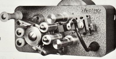
projector. These are rugged double-drum pull-through scanning mechanisms for magnetic reproduction and incorporate a free-running composite sprocket for 35 or 70mm film and easily interchangeable single, four or six track plug in magnetic head assemblies.
