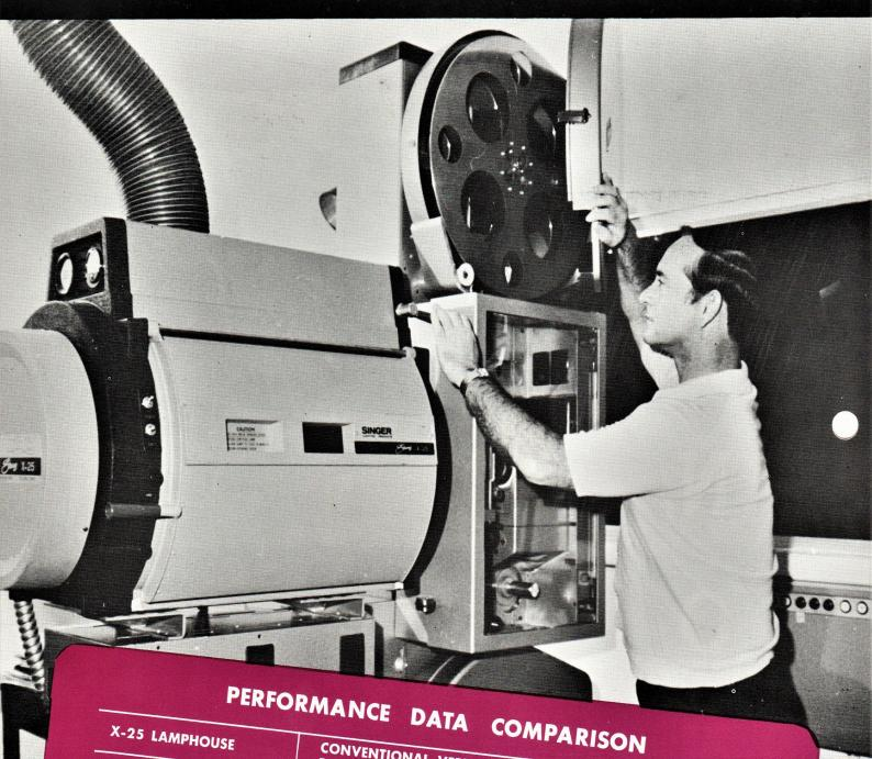
"100" AMP. BULB OPERATING AT 90 AMPS. (Recommended initial current)
