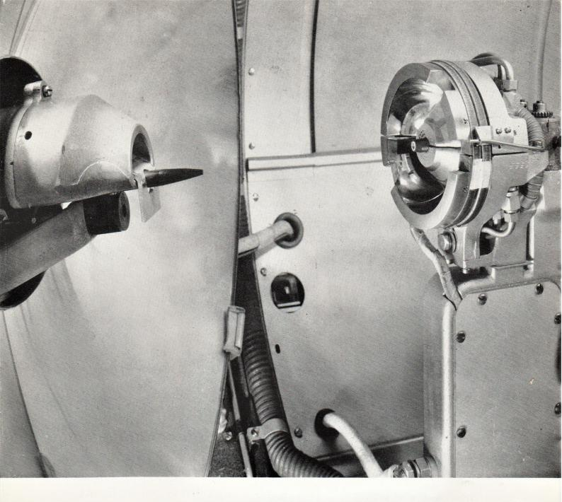
THE 10MM x 27" NON-ROTATING ULTREX positive burns at 140 to 160 amperes and 70 to 78 volts in conjunction with a rotating 7/16" x 12" solid graphite negative carbon. An alternate positive, the 10mm x 25" or 27" Hitex, may be burned at 12.5 to 140 amperes or a 10mm regular positive at 110 to 125 amperes.
