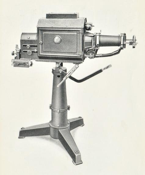
ROSS SPOTLIGHT for Front of House spotting, with Ross Patent Searchlight Arc Lamp in Sheet Steel Lamphouse with & Ellipsoidal Mirror, Automatic Arc Control, Air Blower, Iris Diaphragm and Set of Tinters.
