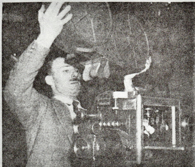
The massive 3-strip mag. weighed 70 lbs loaded. (5 stone or approx 32kg).
