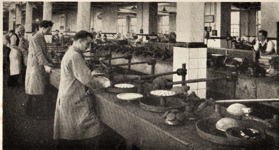
One of the lens polishing shops at Kershaw's factory in Leeds. Note the blocks of polished and unpolished lenses in the right foreground.
