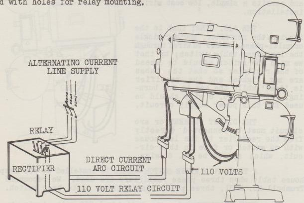
A 30 AMPERE FUSED KNIFE SWITCH should be connected to the alternating supply circuit just ahead of each rectifier so that all of the equipment will be dead when the switches are open.
