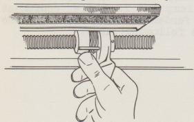
SEPARATE THE CARRIAGES that carry the carbons, to the full limit of their travel, by depressing their spring latches with the thumbs of each hand. This downward pressure will disengage the carriages from the carbon feed screw so that the carriages will slide freely along the carbon feed screw and guide rods.
