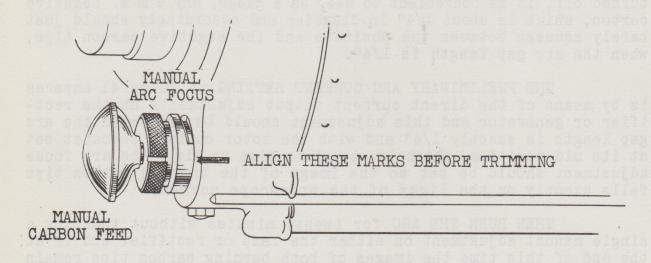
PRELIMINARY ADJUSTMENT OF LIGHT to the screen may be made while the projector is running but without film. However, the final reflector focusing is best done while projecting a picture.
