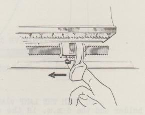
THE ARC should be struck quickly to prevent damage to the arc crater and the possible blowing out of the positive carbon core which might deposit as black soot on the reflector.
