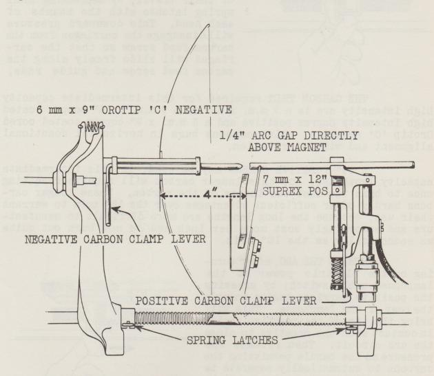
TO TRIM THE LAMP clamp the 7 m.m. carbon in the positive holder and the 6 m.m. in the negative holder. There should be a 1/4" gap between the positive and negative carbon tips and this gap should be directly above the tips of the supplemental magnets. This location of the carbons will assure approximate focus when the arc is first struck.
