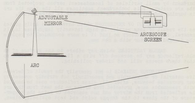
EXACT ARC FOCUS and proper arc gap length are assured after the arcescope has once been set, by simply maintaining the images of the burning carbon tips at these arcescope lines.
