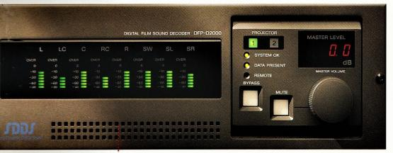
The DFP-D2000 Digital Film Sound Decoder processes digital audio signals, received from the DFP-R2000 Digital Film Sound Reader.
