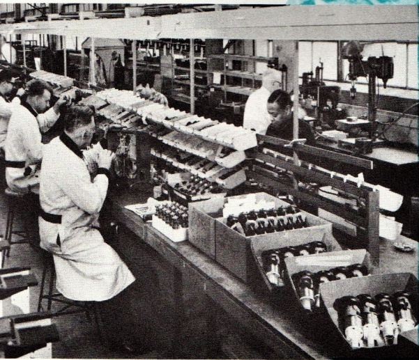
Simplex XL production line where parts and sub-assemblies are added to the main frame.
