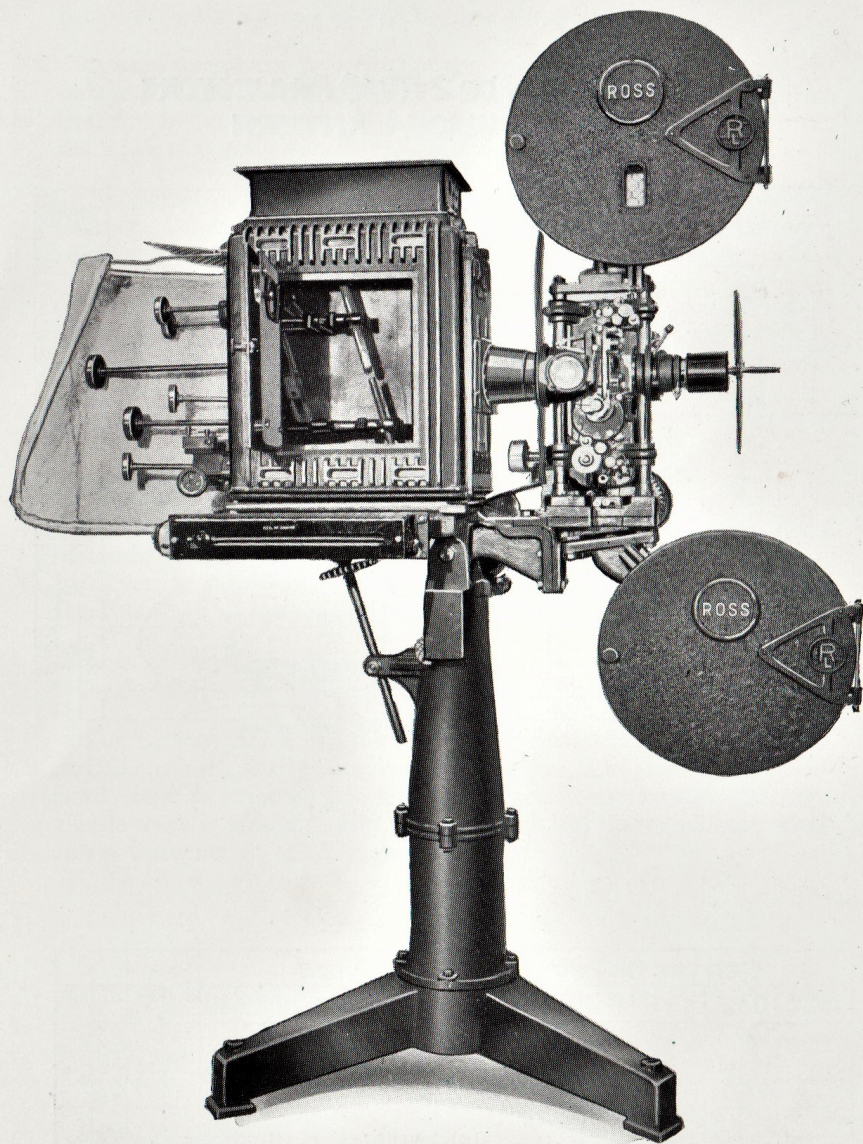
F.C. Model with Aluminium Lamp House and Vertical Arc
