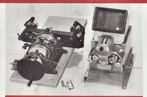
The ideal system for providing level sync. facilities between the "Premier" Synchronisers and standard design front threading Animated Viewers. It avoids offsetting the Viewers and Synchronisers and the consequent difficulties of maintaining Sync. points.
