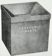
It is a Council Regulation that a receptacle must be provided in a Rewind Room into which all pieces of scrap film can be put. The bin illustrated here meets this Regulation in every respect. The top is fitted with a spring-controlled flap which automatically seals the bin; for emptying purposes the whole top lifts off. It measures  $11'' \times 11'' \times 12''$  deep. Finished in grey crystalline enamel, this bin is a necessity in every Rewind Room.
