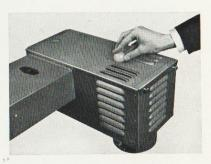
In operation the bingo ball is lifted from the blower unit etc., the number read out and then immediately placed in position for projection.
