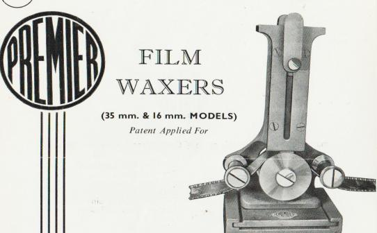
This latest model Film Waxer constitutes a considerable improvement in design and efficiency on all portable Waxers at present manufactured. It is designed for use in Film Processing Laboratories and also in Cinemas showing first run films to apply a thin coating of wax to the edges in order to prevent the emulsion sticking with all the subsequent mutilation hazards during projection.
