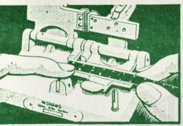
Fit right hand portion of film, emulsion uppermost, on guide pins on right block. Not more than half a frame should project beyond cutting edge.
