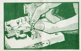
5 Scrape the emulsion from the portion of film projecting from the left clamp (for Automatic Scraper see separate instructions).
