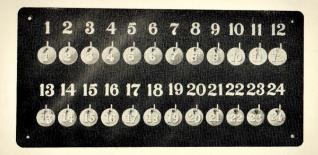
This Disc Board is constructed out of  $\frac{1}{8}$ " thick steel plate and consists of 24 nickel plated steel hooks screwed into the plate and locked behind with hexagon nuts and 24 numbered discs corresponding to the numbers on the Board. 24 spare hooks are supplied for fitting to the Spool Cabinets in the Rewind Room.
