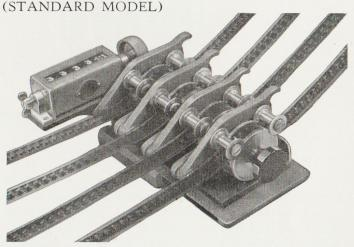
PREMIER 16 mm. Measurers, Frame Counters, Synchronisers are precision made throughout in the best quality materials with all working parts machined to a fine degree of accuracy and allowing for complete protection of the film with specially relieved rollers and sprockets. They are in use in the leading Laboratories and Renting Houses and form essential equipment in progressive Editing Rooms.
