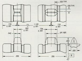
The principal design advantage of the Posi-Trol sprockets is their capability to restrict side movement of the film by means of the sprocket teeth. Compared to standard 35mm sprockets with their .040" or .055" wide teeth, Posi-Trol sprockets have one row of teeth that nearly matches the .110" wide film perforations, virtually eliminating lateral slippage. This acts to stabilize the image on the film in a camera, or the projected image on the theater screen.
