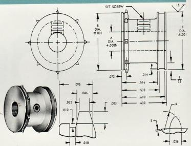
machined from type 303 non-magnetic stainless steel, except 208B25F which is machined from type 416 stainless steel. The 208B25F sprocket includes two set screws  $90^{\circ}$  from each other.
