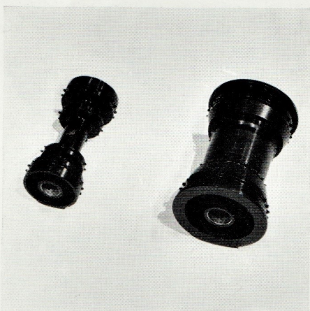
Fig. 6. The sprockets with two rims for 35-mm film and two rims for 70-mm film.
