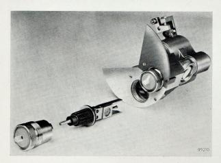
The lamphouse is equipped with an automatic waterflow relay and a magnetic water lock. The former prevents the lamp from being switched on when the water supply is insufficient, the latter closes the water circuit when the lamp is not in use, thus avoiding needless water consumption.
