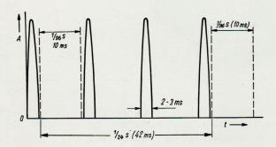
The dark periods are sufficiently long to permit of the use of a normal intermittent system with a  $90^\circ$  Maltese cross. No rotary shutter is required. All the light produced is completely utilised for projection instead of about half of it being lost because of the shutter. The lamp, operated at 800 W, produces the same luminous flux as a H.I.-arc of 60 A.
