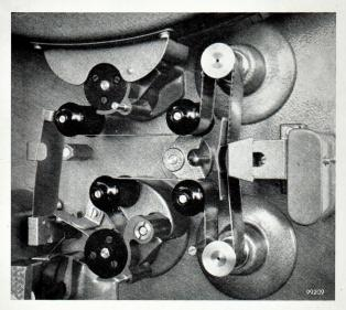
The magnetic soundhead has two sound drums, running in precision ball-bearings and provided with heavy flywheels, and a head assembly for one-to-four track reproduction. When a magnetic soundhead is used, the projector is equipped with two feed sprockets, the upper one for pulling the film from the reel and the lower one for pulling it through the soundhead.
