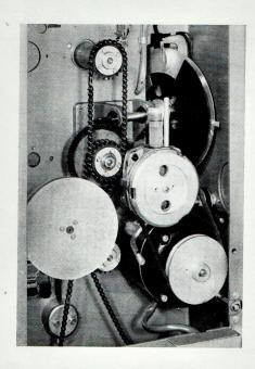
The new framing device requires no phase correction and hence no gear transmission for this purpose. All the spindles and shafts run in sealed ballbearings, requiring no lubrication, and all the guide rollers are made of self-lubricating material.
