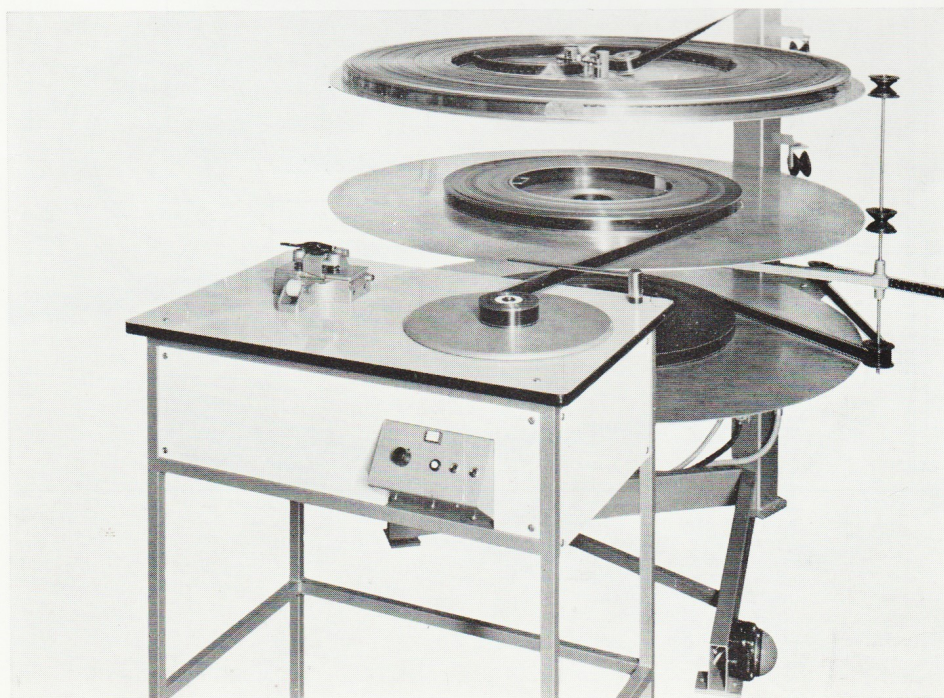
Programme 1 being screened and programme 2 being prepared at the same time. The item to the left of the winding disc is a tape splicer.
