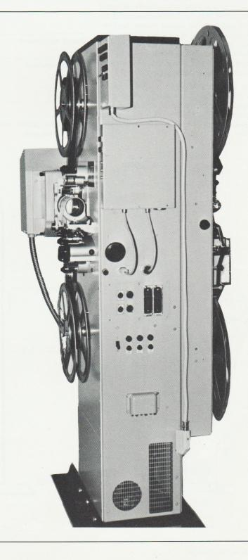
The projector FP 38 is formed by a column-shaped cabinet provided with a hinged door. The column and the 35 mm part of the projector FP 38 which it accomodates, are identical to the well-known projector FP 30. The front supports on easily interchangeable panels the projector mechanism with the optical sound head, the two frictions, the lens holder or turret, and – on request – an additional 4-track magnetic sound head.
