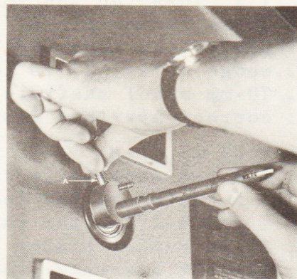
Fig. 5 Removal of spool shafts
