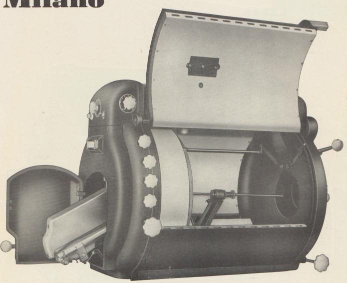
Vernier adjustment of mirror and negative-carbon positioning, and of differential carbon feed.
