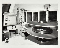
Film travels from one of the RotoMatic discs through either of two projectors. Film is projected and returns to take-up disc ready for rethreading through projector at end of show. Only simple interchange of supply and take-up plug-in units and re-setting control unit functions is required between shows. Film need never be rewound or removed from discs.
