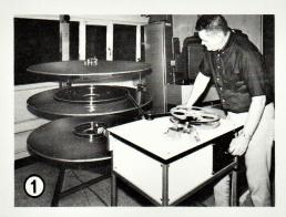
Operator makes up program by loading film from exchange reels onto the system from Program Table. Up to  $4\frac{1}{2}$  hours of film may be loaded on a single disc. This loading procedure generally takes place at the beginning of a run and does not have to be repeated until a new program is being prepared. However, with Roto-Matic a new or special program may be loaded even during show, using free disc.
