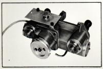
Servicing the DP-75 is quick and uncomplicated. This heavy aluminum casing contains seven helical cut steel gears in an oil filled enclosure. Prefitted parts can be replaced with a screw driver and a wrench.
