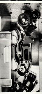
New anti-buckle film gate\* construction is a feature of the Norelco Universal DP-75 projector. It prevents heat flutter and defocusing without necessity for cumbersome air pressure devices or liquid gates sometimes found when very powerful light sources
