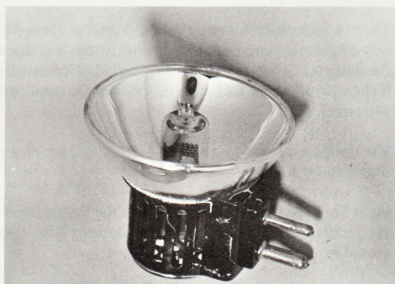
Typical of the lamps used in current 16mm portable projectors is the 24V, 250W tungsten halogen EMM. It has a pre-aligned dichroic reflector directing visible radiation forward and allowing a high proportion of infra red to escape to the rear.
