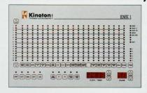
What makes the EMK1 electronically controlled system stand out is the large number of functions, the ability to preset sound levels and the brightness of the auditorium lighting. and not least the storage of 6 different complete programs.
