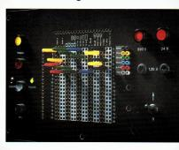
For decades Kinoton's matrix automation has proven its worth. It is available in two versions: built into the projector or wall mounted. Controlled by foils on the film print, the matrix programmer reliably controls the auditorium's program as preset on the matrix.
