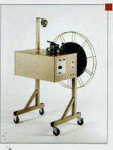
The MUU 2000 make-up unit is the ideal economical accessory for our non-rewind systems. Fast make-up and tear-down speeds can be reached with the proven drive system used in our MT/UT tables. The vertical layout results in a more compact unit. Standard features include electronic speed regulation, reversible shaft rotation and automatic film run-out switch.
