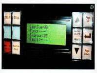
The CCA 3 offers 7 program routines for projector control and auditorium functions. 3 sensors on the projector detect metal cue foils on the film and start the program routines. The CCA3 is a comfortable and versatile system, allowing interlock operation and additional functions by expansion modules.
