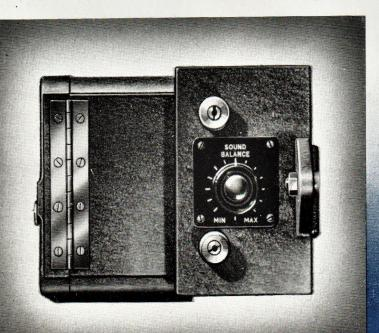
This control rheostat mounted on the forward end of the soundhead frame regulates the brightness of the exciter lamp. The accurate matching of sound level between the two machines at change-over is thus conveniently and instantly assured.
