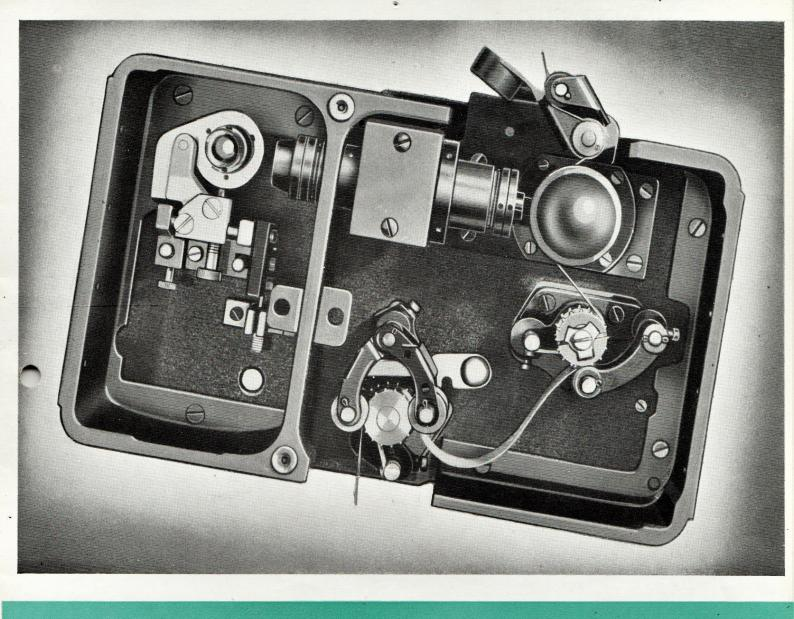
An extra lamp and holder is supplied ready for immediate use should the lamp fail in operation. A safeguard against failure is provided for by deliberately arranging that the lamp is under-run.
