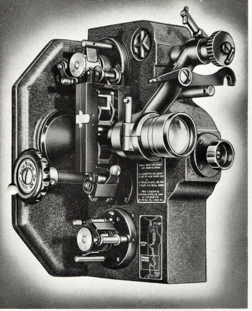
The two-bladed rear shutter runs in a substantial totally enclosed guard. A safety shutter of the flag type, governor controlled, works in front of the rear shutter and comes into action as soon as the speed of the machine falls below a predetermined limit. This action cuts off light and heat from the film in the event of any stoppage of the mechanism, thus preventing fire.
