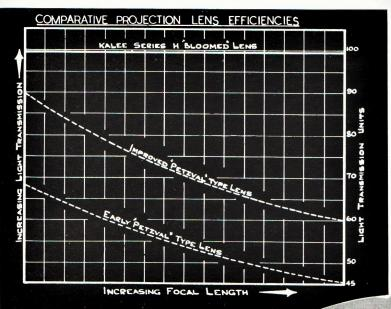
The whole range of Kalee Series "H" projection lenses possess a constant F value. This means that each lens, whatever its focal length, passes the same maximum amount of light to the screen, as is graphically illustrated by the straight line characteristic in the chart. This feature of constant F value results in an appreciable gain of illumination.
