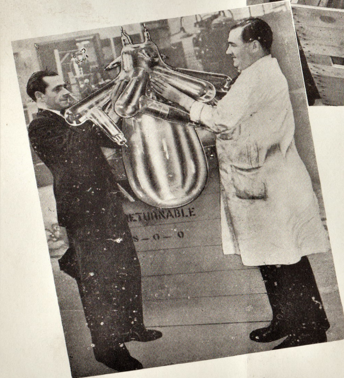
Fig. 2. Typical method of suspension-packing of a Nevelin standard 6-arm bulb. Untying the webbing knots leaves the bulb suspended in its under-seating. (Section 3 (b).)
