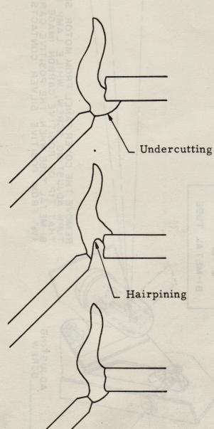
"UNDERCUTTING" of the arc flame is caused when the negative carbon is adjusted too low. Raise the negative carbon by turning the turnbuckle nut of the adjusting rod counter-clockwise.
