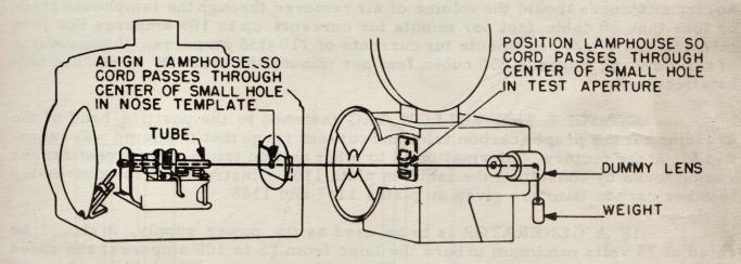
ONE ALIGNING KIT NUMBER 23481 is supplied with each pair of lamphouses to provide an accurate and reliable method of locating the lamphouse on the projector base, so that the ultimate in optical efficiency and screen illumination can be obtained.
