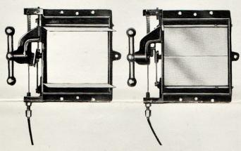
A simple and trouble-free mechanism to obtain the perfect change-over. It consists of two frames fitted with shutters, which are linked by Bowden cable. Finger touch of the control knob on either frame instantaneously closes one shutter and opens the other. Easily fitted to any make or type of projector.
