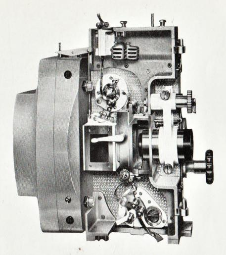
The Gaumont-Kalee '19' and '20' Projectors, similar to above illustration, are equipped with the normal two-blade shutter. Model '19' does not embody an electrically-operated change-over device.
