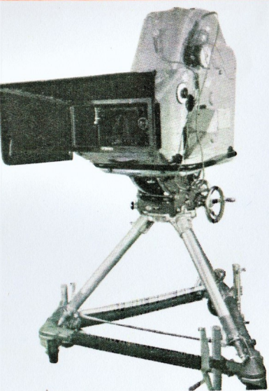
Studio type Technirama camera showing new blimp which weighs only 170 lbs. This camera is fitted with 2,000 ft. magazines.
