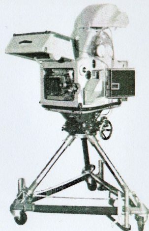
Studio type Technirama camera showing new blimp with the various doors open giving access to the camera for lens change, re-loading, etc.
