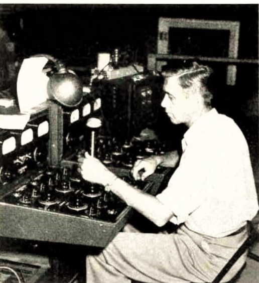
The "mixing" console from which the sound from the six individual "pick-up" microphones is controlled on its way to the six magnetic-type tracks.
