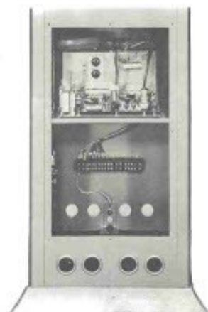
JIL 11 Pedestal-and-column arrangement with lower cover removed. The upper frame contains the pre-amplifier, the lower one houses electrical connections; the middle frame contains the A.C. connections; left edge: D.C. connections for xenon lamp.
