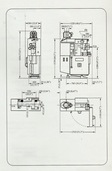
Bauer U 3 with 4 or 6.5 KW lamphouse. With 0.9—2.5 KW lamphouse, overall height 1560 mm (61.3")
