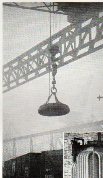
Fig. 43.—Magnetic chuck operated by an air-cooled Westalite rectifier.
