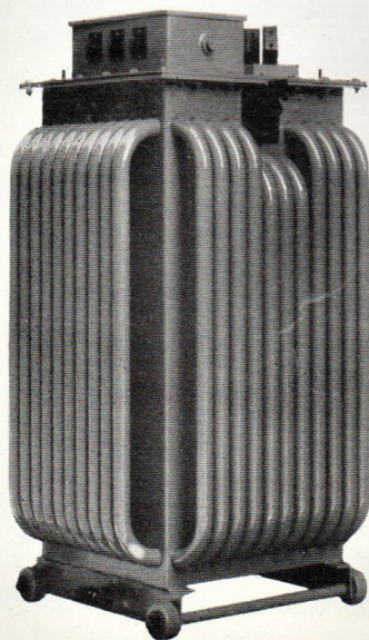
Fig. 52.—Typical plating rectifier with 63-step control included in the same tank as the main transformer and rectifier. Output 7.5 volts at 1,000 amperes.
