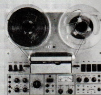
The first licensed consumer product with Dolby B-type NR: the KLH Model 40 recorder.
